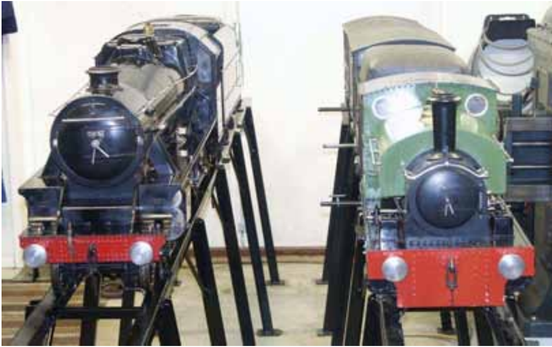
Figure 7: The Stanier Black Five and Jonas Bagge standing side by side in the workshop. Note the saddle tank and the small boiler of Jonas Bagge.
