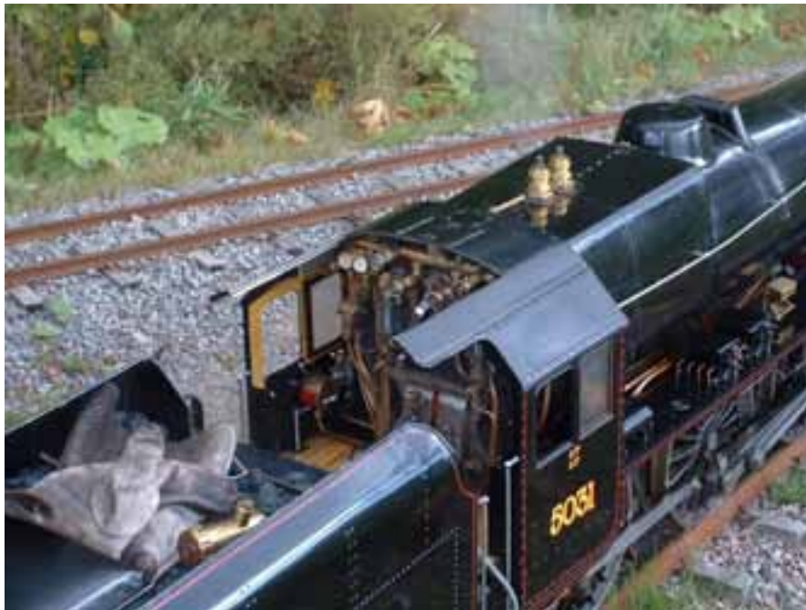
Figure 6: Close up of the Black Five cabin. Seen are the steam and vacuum (painted red) brake controls and the gauges showing degree of steam pressure and vacuum. The slit in the fire doors reveals the glow of the fire. In the tender lies the electric booster control.
