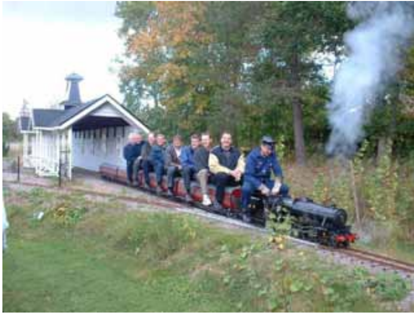
Figure 5: The Stanier Black Five and the LMS scale coaches pulling out of the terminus station on a cold autumn day (seen by the amount of steam condensation). The first coach is equipped with an electric motor booster to support operation in rainy weather.
