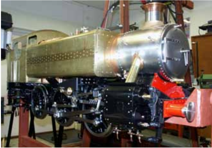
Figure 8: The 1500 class engine model. The relatively large dimensions of boiler and cylinders are evident.
