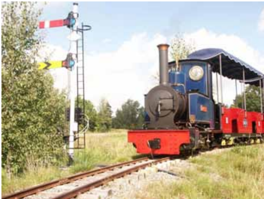
Figure 3: The stop (red wing) and distant (yellow wing) semaphore signals are distantly operated by computer controlled electromechanical servos. The plastic tubing for communication and illumination power cables is plainly seen. In the photo the engine is Brasken pulling empty coaches complete with their smoke protecting canopies.
