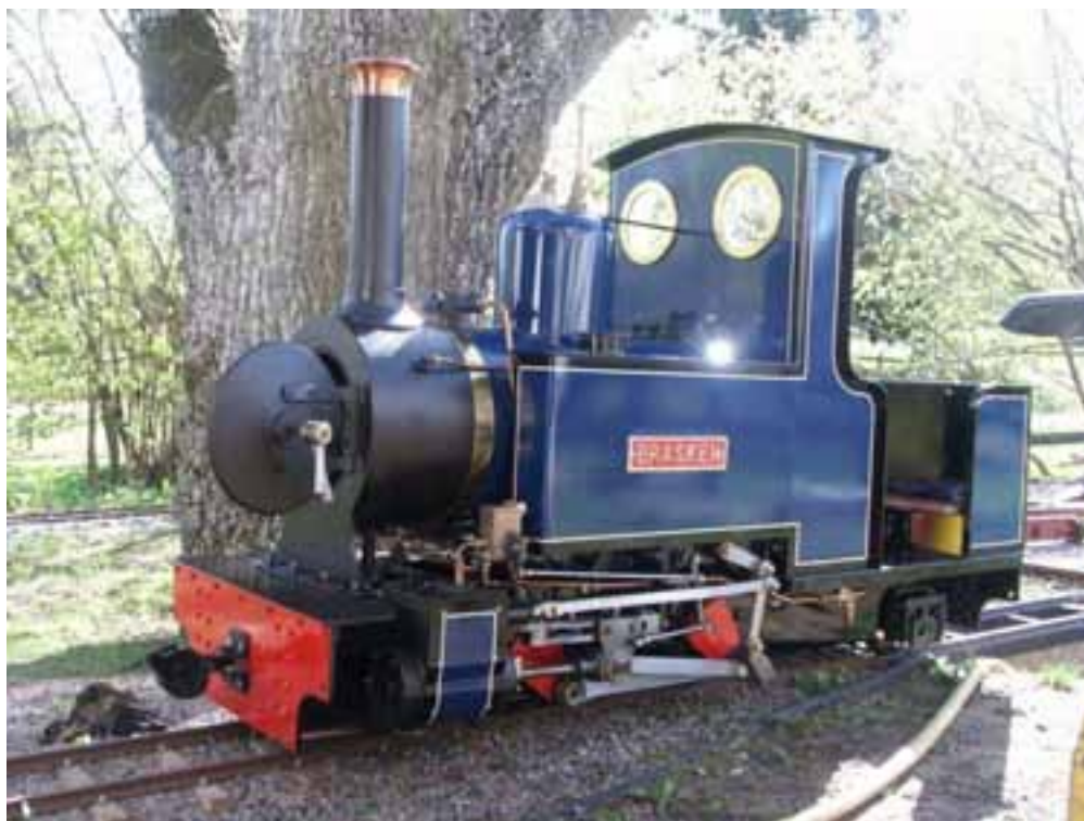
Figure 11: Brasken being cleaned outside its shed. Note the arrangement with outside frames and cranks. The valve gear is of Marshall type, also characteristic for well-known Ornstein and Koppel narrow gauge engines. It has the advantage of avoiding the complexity of an expansion link, present in most other valve gears.
